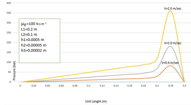
Fig. 2, effect of Drawing Speed on Pressure Distribution within the Unit
