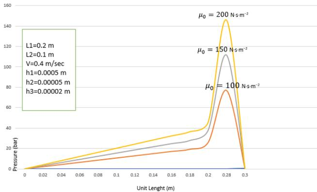
**Fig. 4, effect change  $\mu_0$  (initial viscosity) on pressure distribution and maximum pressure within the unit**
