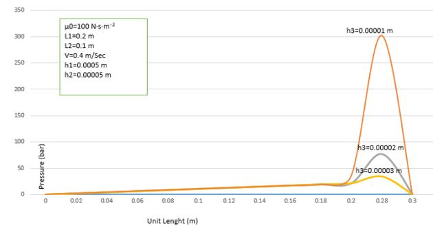
Fig. 3, effect of outlet gap ( $h_3$ ) on pressure distribution within the unit
