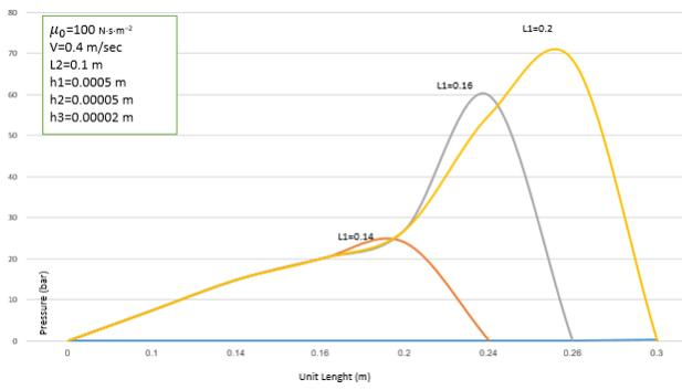
**Fig. 5, effect change of  $L_1$  on pressure distribution and maximum pressure within the unit**
