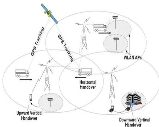
Fig.1, Horizontal and vertical handoff for heterogeneous network
