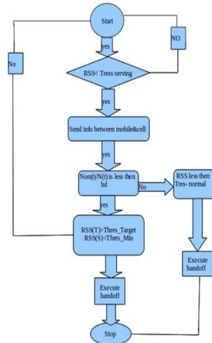
Fig. 2, adaptive algorithm
