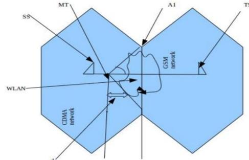
**Fig.3, Analysis of probability of handoff failure & initiation as mobile moves from Ss to Ts via WLAN**
