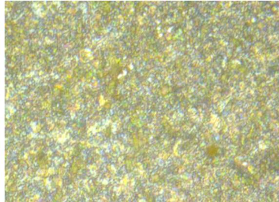
Fig. 5 Optical micrographs of the AISI 410 microstructure developed by austenitization treatment at 860°C for 24 min followed by furnace cooling to room temperature “annealing”. Picric etch.
