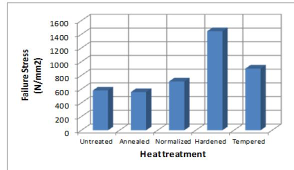
Fig. 9 Tensile strength of treated and untreated samples of AISI 410 martensitic stainless steel.
