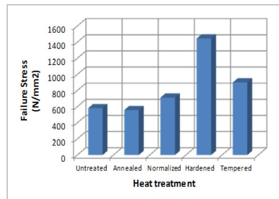
Fig. 11 Failure stress of treated and untreated samples of AISI 410 martensitic stainless steel.
