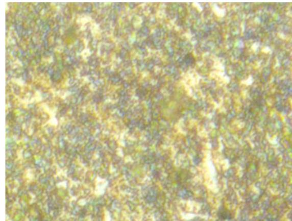
Fig. 6: Optical micrographs of the AISI 410 microstructure developed by austenitization treatment at 920°C for 1 hour followed by air cooling to room temperature “normalizing”. Picric etch
