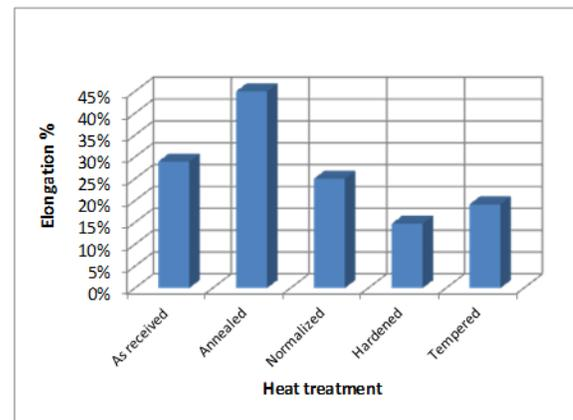
Fig. 10 Percentage elongation of treated and untreated samples of AISI 410 martensitic stainless steel.
