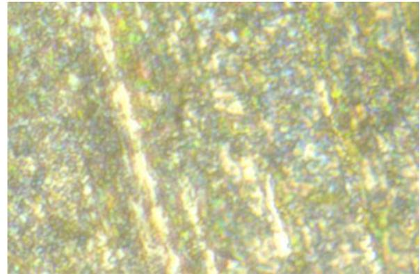
**Fig. 8 Optical micrographs of the AISI 410 microstructure developed by austenitization treatment at 972°C for 30 min followed by oil quenching to room temperature then tempered for 1 hour at 510°C and air cooled. Picric etch**
